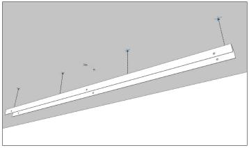
Step 1: Offer back strap bracket to ceiling to mark where fixing holes will be located.
