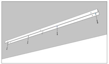
Step 2: Bring mains feed though centre hole and secure back strap to ceiling using suitable fixings.
