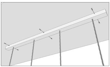
Step 5: Ensuring that no wires are trapped, offer ceiling bar up to back strap and secure using supplied machine screws.
