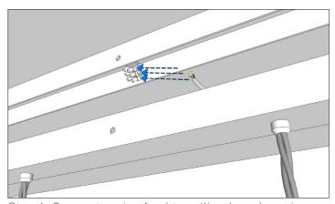
Step 4: Connect mains feed to ceiling bar observing polarity.
