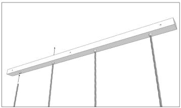
Step 3: Thread flex from lights through cord grips on ceiling bar. Wire into loom observing polarity. Set pendant height and tighten cord grip.
